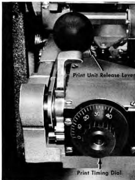
Figure 201. Print-Timing Dial and Print-Unit Release Lever
